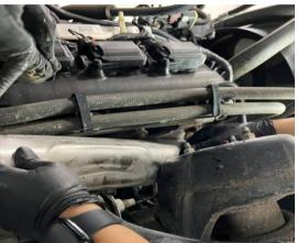
Use size **10 mm & 13 mm** socket to undo the bolts securing the manifold to the vehicle.
