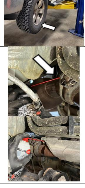
Remove the 4 flange bolts from passenger and driver side manifold to collector flange using **9/16 in** socket.
