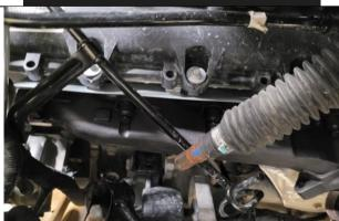
Position the manifold with the gasket into place and install the supplied M8 bolts along with supplied spacer (1403009).
