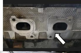
Set the manifold into position, then slide the corresponding gasket between the manifold and cylinder head.
