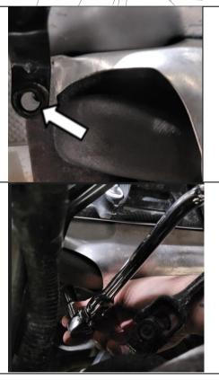
Using **10 mm & 13 mm** socket, remove the left side exhaust manifold bolts. Remove the manifold and gasket carefully
