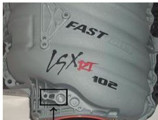
Intake Mounted Purge Valves
