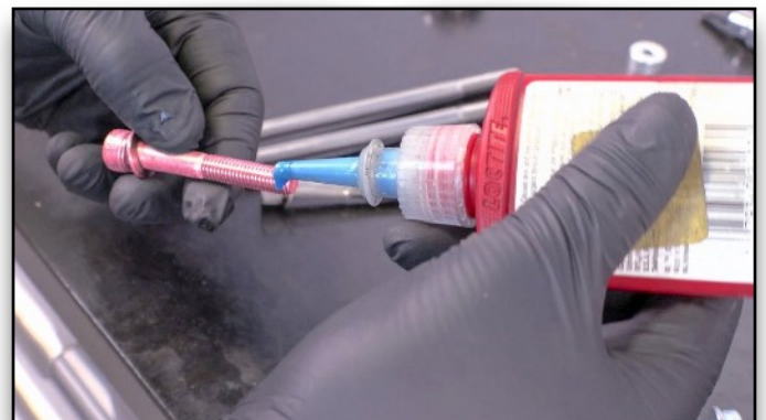
81. Place Washers On Hex Cap Crews. Apple Some Blue Thread-locker As You Install Them
