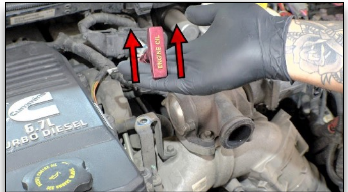
32. Bend Tube Up Slightly
