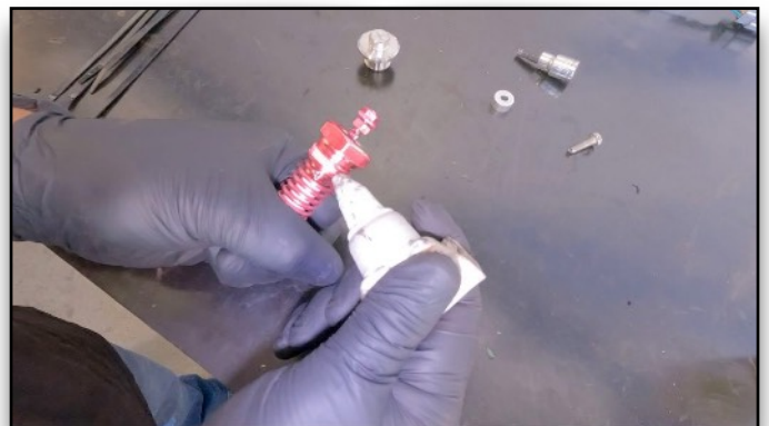
105. Apple Sealant To Heater Coil
