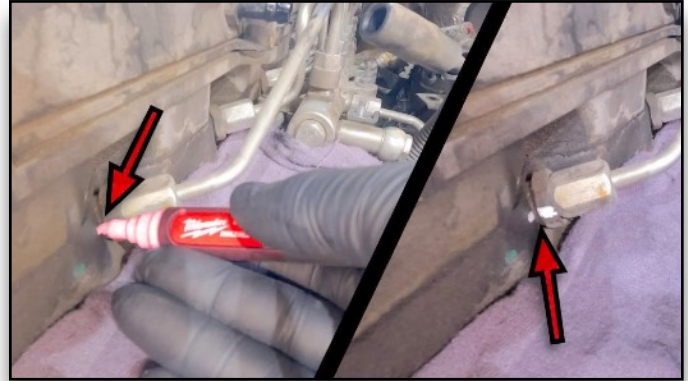
55. Paint Marker Line Across Threaded Insert & Cylinder head
