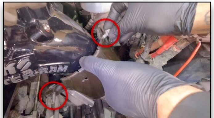
125. Install Throttle Heat Shield Bolt & Nuts
