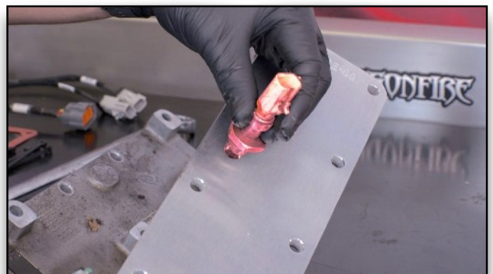
67. Transfer Temp Sensor to Banks Plate
