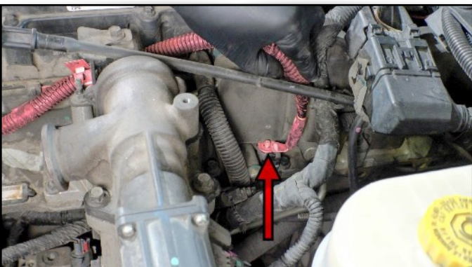
30. Remove Heater cable from Terminal
