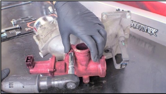
68. Remove EGR Valve & Throttle
