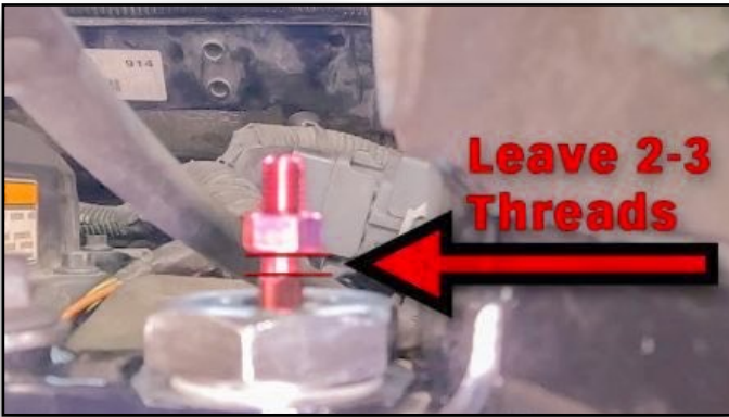
114. Apply Red Thread Locker to Coil Heater
