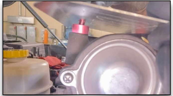
123. Place Rear Heat-shield Spacer & Screw
