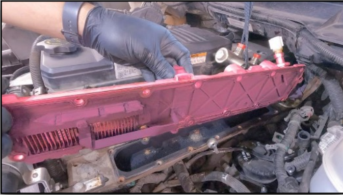
63. Remove Factory Grid Heater
