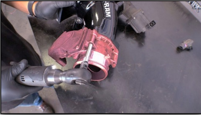
76. Fasten Throttle Body to Monster-Ram
