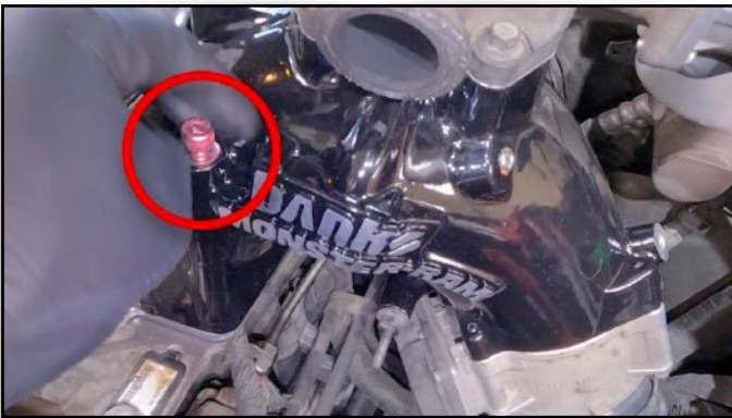
103. Put Long Bolt Into Front Corner by Hand
