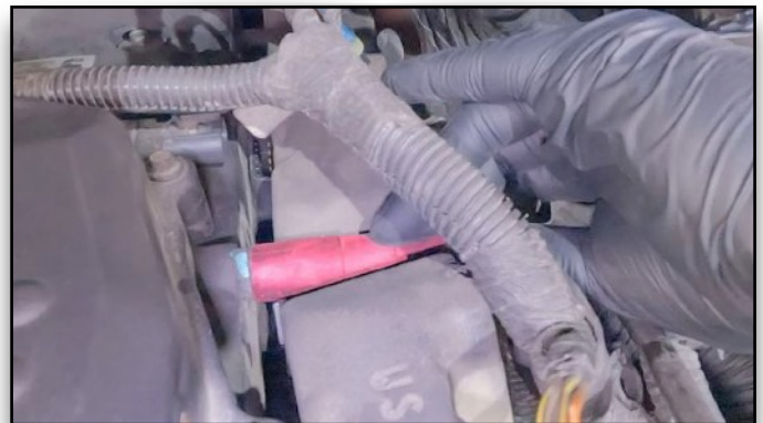
94. Connect Rear PCV Hose Back To Valve Cover
