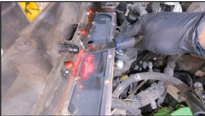
64. Clean Manifold Surface
