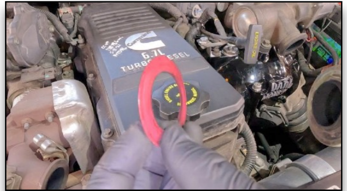
116. Flat Washer Goes on Passenger Side of EGR Tube
