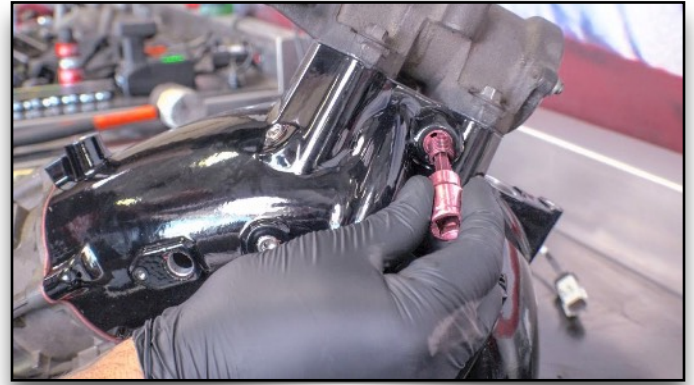
78. Install Rear Thermocouple Plug
