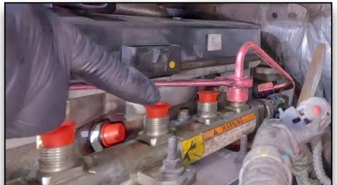
87. Tighten Fuel Lines to 41 ft/lbs
