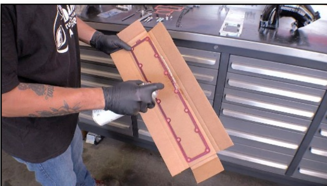
65. Spray Adhesive to Gasket (Banks Side)
