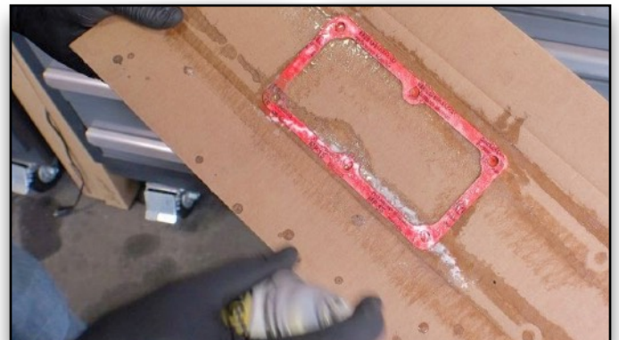
80. Spray Gasket With Adhesive
