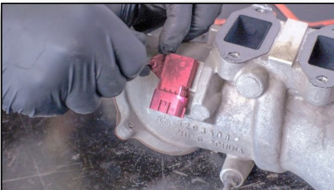
70. Remove & Transfer MAP Sensor
