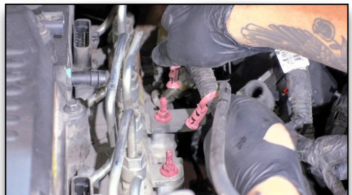
50. Remove Cable Ties from Driver Side Studs
