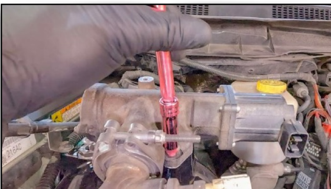
121. Loosen Front Bolts on EGR Cover
