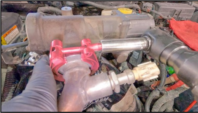
119. Tighten Driver Side Clamp
