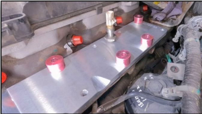
83. Place Fuel Rail Standoffs
