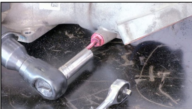
71. Remove & Transfer Elbow Stud
