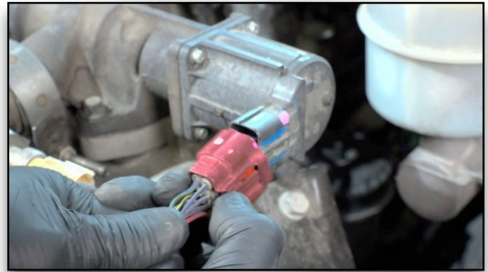
18. Remove EGR Valve Plug Press the locking tab, press the plug forward to release tension, then pull back to remove.
