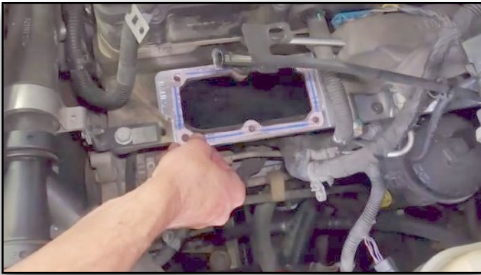
82. Hold Billet Plate In Place w/ Stock Bolt
