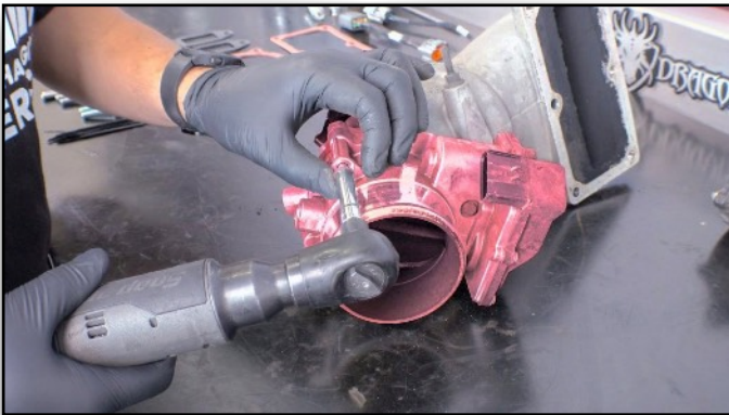
69. Remove Throttle Body
