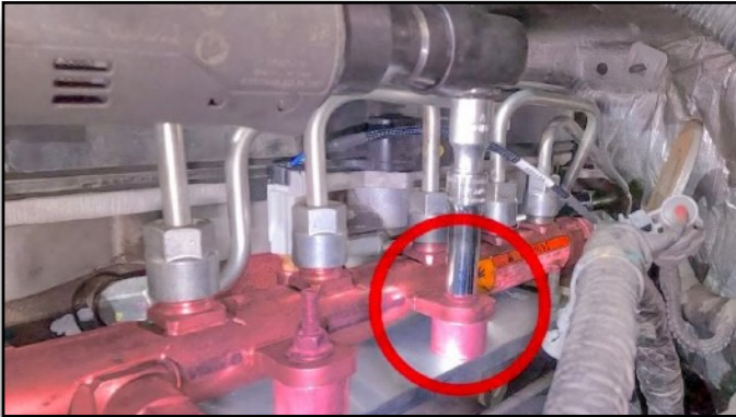
90. Remove Middle Right Stud For Dipstick Tube
