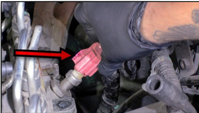
53. Remove Manifold Temp Sensor Plug
