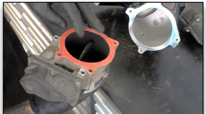
75. Align Throttle Body Gasket
