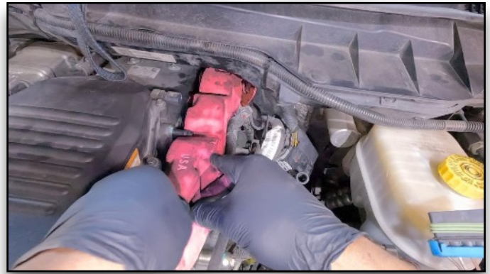
92. Put Rubber Isolator Back Into Place
