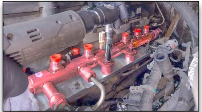
86. Tighten Fuel Rail
