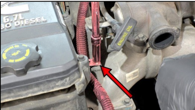
29. Remove 12V Harness P-Clamp
