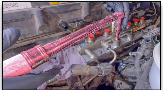
Torque Bolts to 18-20 ft/lbs
