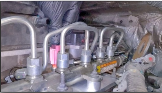
89. Connect Temp Sensor Extension Harness Be sure to lock the plug once connected.
