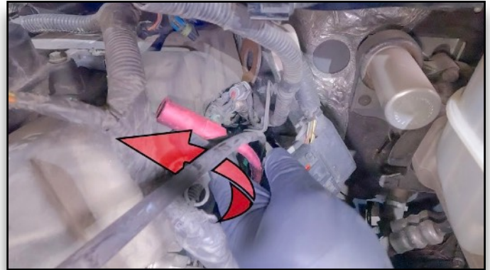
93. Run Rear RCV Hose Under Dipstick Tube
