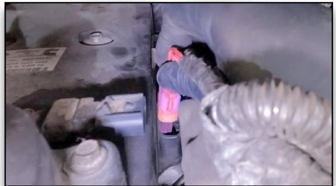
95. Connect Rear Flat Blue Injector Plug
