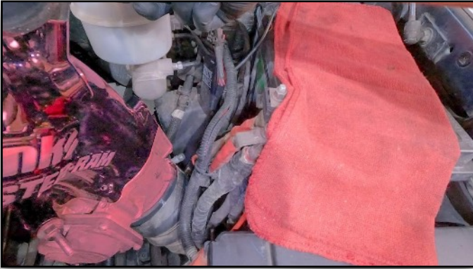
102. Insert Monster-Ram Into Boost Tube
