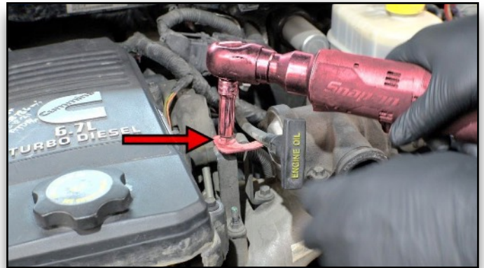
31. Remove Dipstick Tube Bracket
