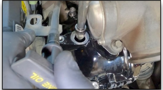
Use Hex Key Extension to Tighten Bolt
