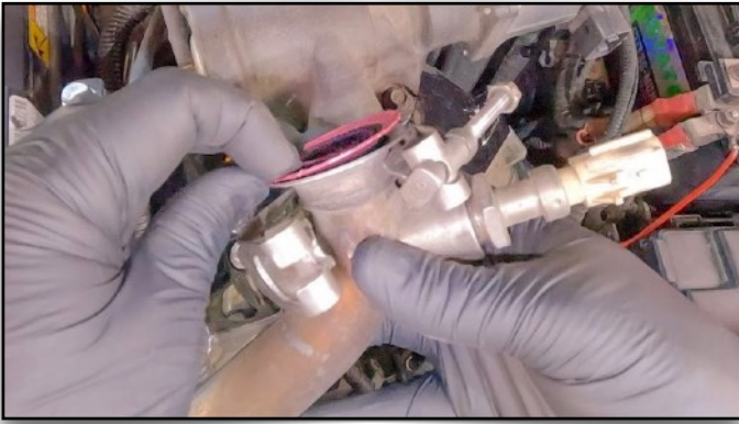
118. Conical Gasket Goes On Driver Side of EGR Tube
