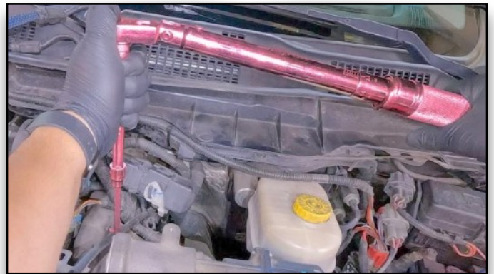
Tighten All Bolts to 18-20 ft/lbs
