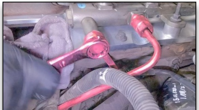
88. Tighten Fuel Supply Line Banjo Bolt Hand Tight. Tighten Fuel Feed Line to 41ft/lb
