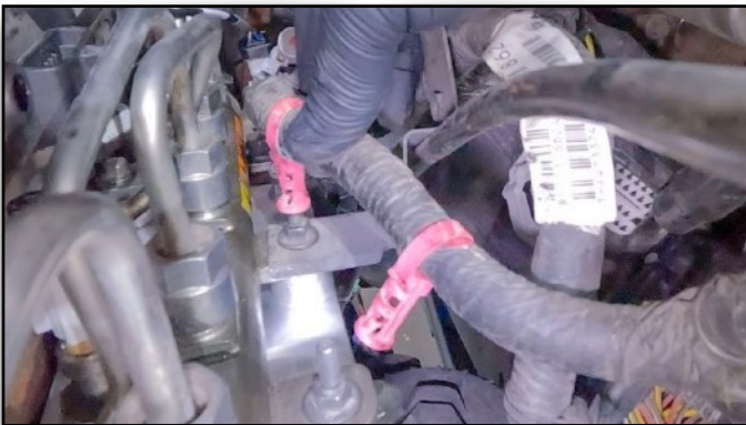
91. Push Engine Harness Cable Ties Back Onto Studs
