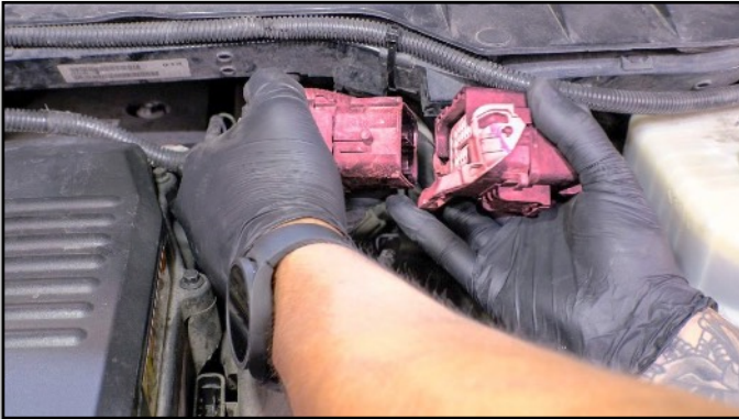
45. Disconnect Large Driver Side Engine Harness
