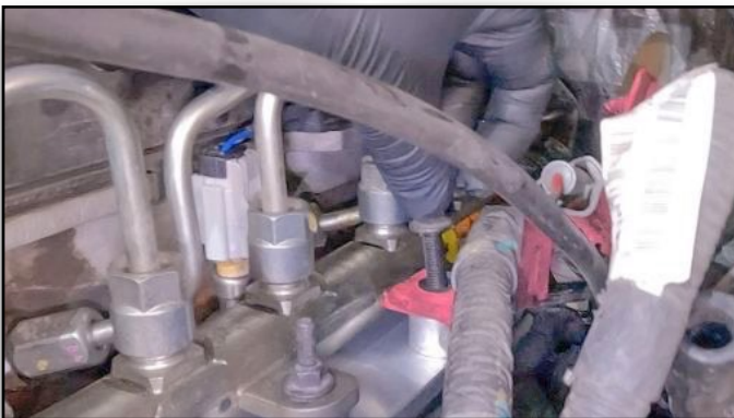
Slide Dipstick Bracket Over & Reinstall Stud
