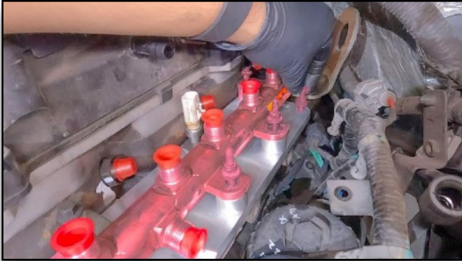
84. Release Bungee Cord. Place Fuel Rail & Studs in Place
