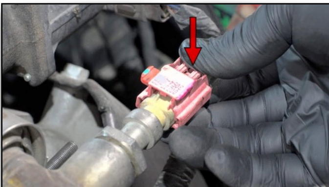
17. Remove Temp Sensor by Pinching It
