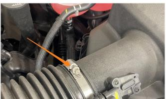
3. Remove the PCV line from the passenger side valve cover by pressing in the grey tab and pulling away from the engine. Remove the PCV line from the intake manifold in a similar fashion and remove the line from the vehicle. It may be helpful to remove the ignition coil electrical connector next to the intake manifold fitting for easier removal. If you have a 6.2L engine, the intake manifold fitting will be located just above the throttle body.
