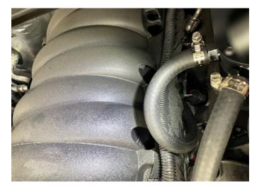
**8.**Take the hose with the straight fitting and install the quick connect fitting to the fitting on the valve cover. Attach the open side of the hose to the "IN" fitting on of the catch can and secure with included worm gear clamp. The worm gear clamp is optional and the catch can will function leak free without the clamp. (Image on Top Right)
