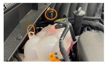
5. Ilnstall the 2x included fittings onto the catch can with a 17mm wrench. Then, secure the catch can to the bracket with the included M4 bolts, as shown. Do not fully tighten the bolts so that the assembly can be adjusted later.
