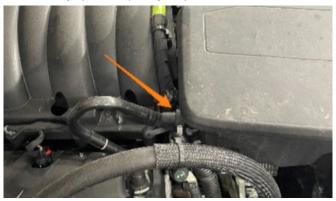
2. With a 7mm socket or flathead, loosen the 2x clamps on the intake assembly. The first clamp is located behind the mass air flow sensor and the second clamp is located at the throttle body. Remove the intake from the throttle body and mass air flow sensor and rotate the intake assembly counter-clockwise out of the way.
