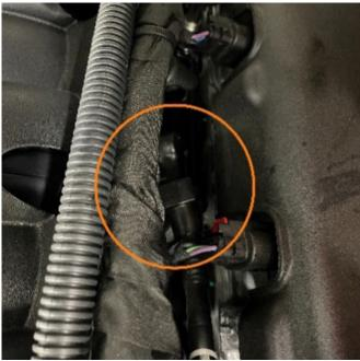
**4.** Remove the 1x 10mm bolt securing the coolant reservoir to the vehicle. Remove the reservoir off the studs on the firewall but do not attempt to remove it from the vehicle.
