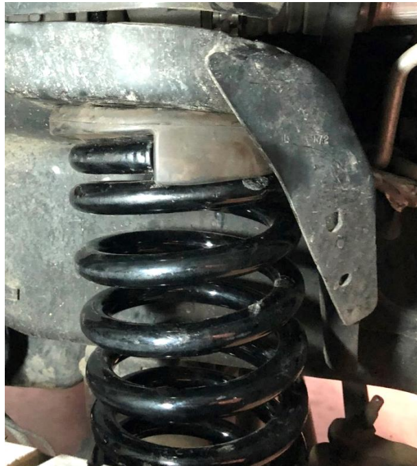
Figure 2. Synergy Leveling Spring Installed - Spring Isolator Not Fully Seated
