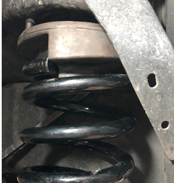
Figure 2. Synergy Lift Spring Installed - Spring Isolator Not Fully Seated
