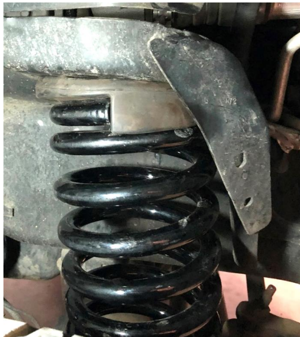
Figure 3. Synergy Lift Spring Installed - Upper Spring Isolator Correctly Seated
